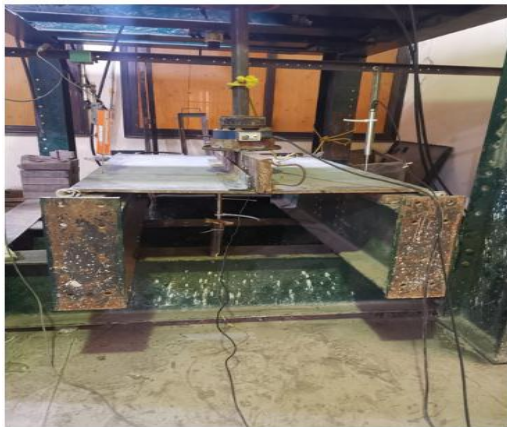
Figure 2. Three points loading flexure test setup
